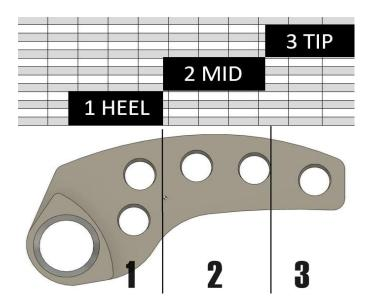
You can start adjusting from the image below. Don't be overly concerned about exat weight placement at this time, it's only starting point. Your machine should run in most cases 7000-7400rpm.
