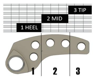
You can start adjusting from the image below. Don't be overly concerned about exat weight placement at this time, it's only starting point. Your machine should run in most cases 7000-7400rpm.
